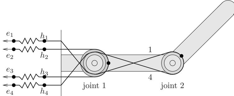
Figure 6.10: Planar finger with position-controlled elastic tendons.
