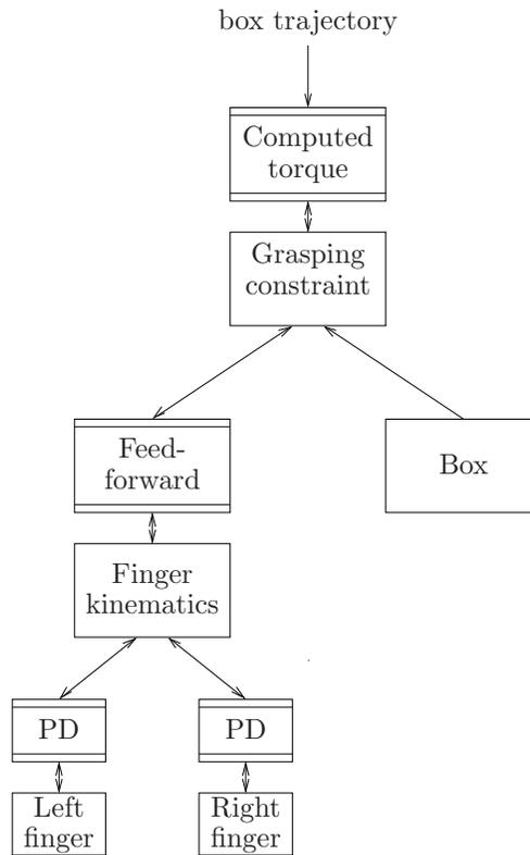
Figure 6.15: A hierarchical controller for multifingered grasping.
