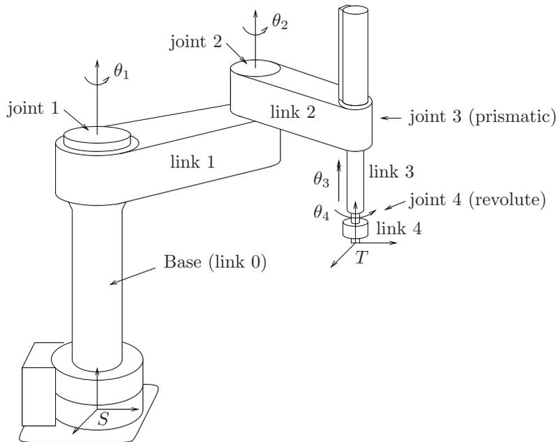
Figure 3.1: Numbering conventions for an AdeptOne robot.
