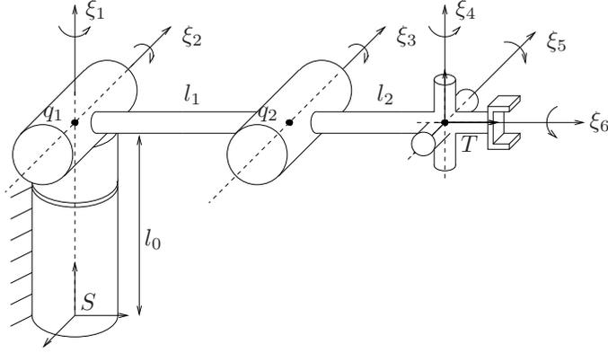
Figure 3.4: Elbow manipulator.
