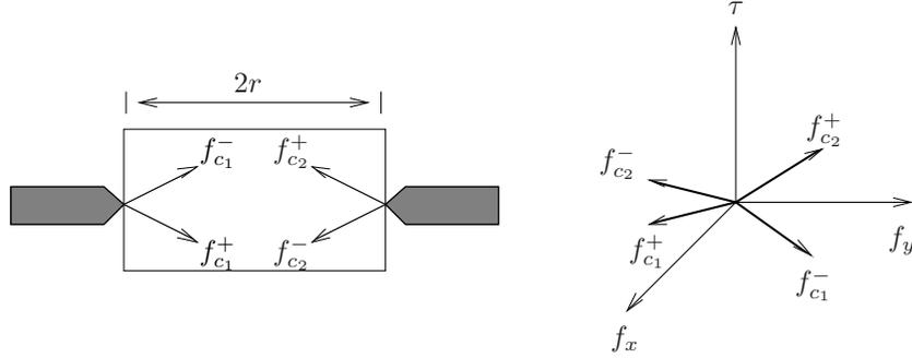
Figure 5.9: Force-closure for point contact with friction.
