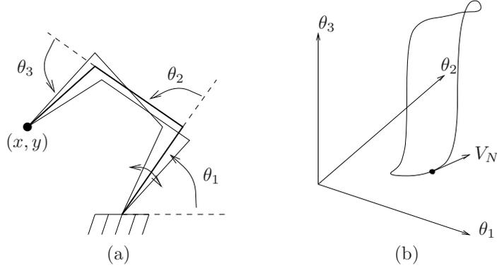
Figure 3.17: Self-motion manifold for a redundant planar manipulator.
