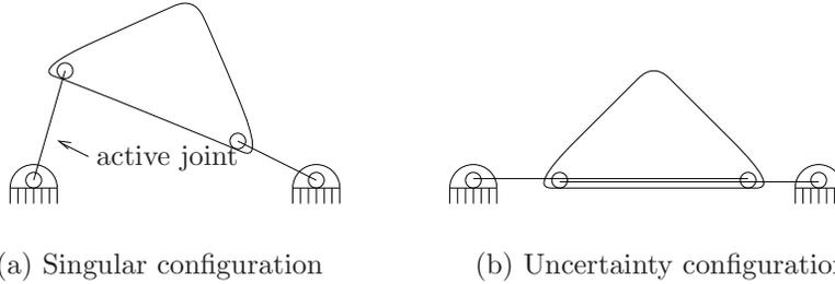
Figure 3.20: Potential singular configurations for four-bar mechanisms.
