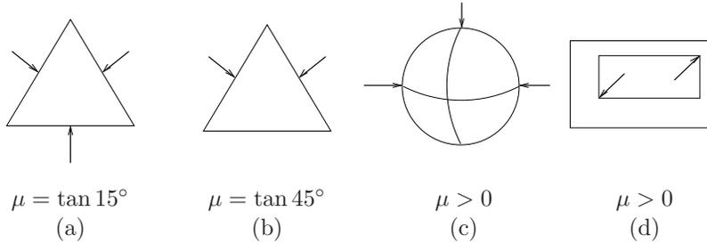
3. Construct the grasp map for the grasps shown below and write the friction cone conditions with respect to the contact basis you choose. Determine if the grasp is force-closure. Assume that all contacts are soft-finger contacts.
