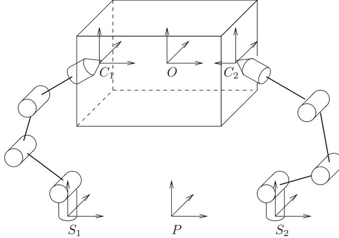
Figure 2.14: Coordinate frames for a simple grasping example.
