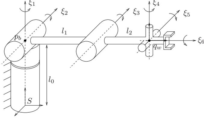
Figure 3.11: Elbow manipulator.
