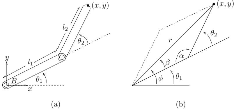
Figure 3.7: Inverse kinematics of a planar two-link manipulator.
