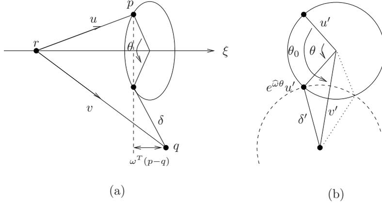
Figure 3.10: Subproblem 3: (a) Rotate  $p$  about the axis of  $\xi$  until it is a distance  $\delta$  from  $q$ . (b) The projection onto the plane perpendicular to the axis. The dashed line is the “flip” solution.
