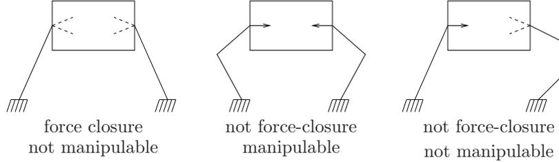
Figure 5.16: Some grasps illustrating manipulability and force-closure properties.
