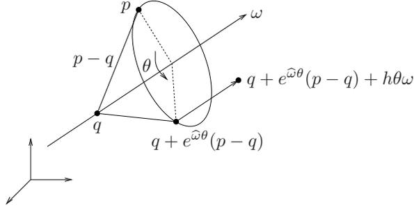
Figure 2.8: Generalized screw motion (with nonzero rotation).
