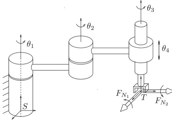
Figure 3.15: End-effector wrenches which generate no joint torques.
