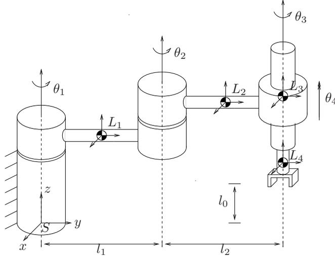
Figure 4.6: SCARA manipulator in its reference configuration.
