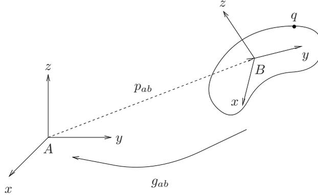
Figure 2.3: Coordinate frames for specifying rigid motions.
