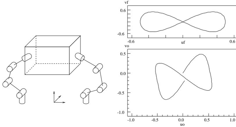
Figure 8.3: Steering applied to a multifingered hand.
