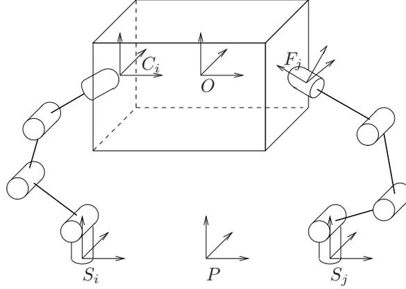
Figure 5.24: Grasp coordinate frames for moving contacts.
