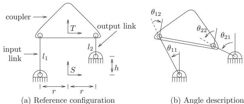
Figure 3.19: Four-bar linkage.
